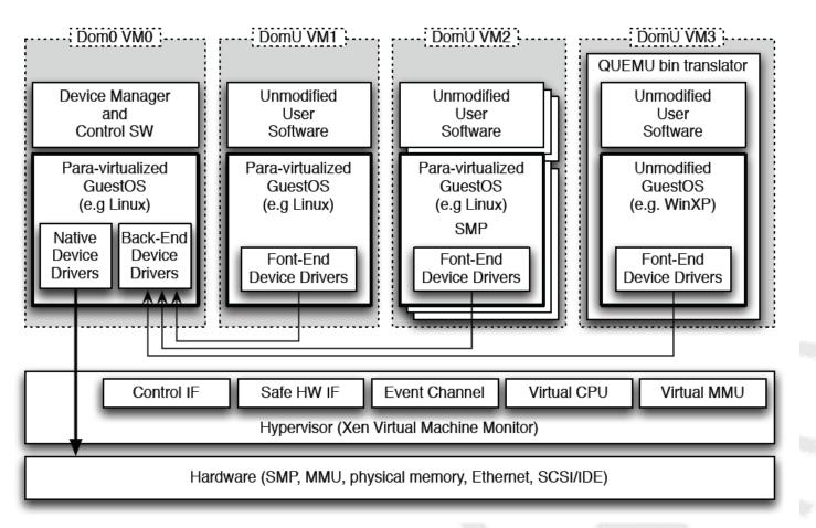
A physical node running 3 VMs (2 to 3 VCs nodes. One runs Windows through QUEMU). Xen provides the virtualization
